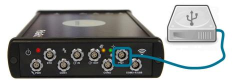
Figure 4-20: Connecting an external USB memory device to the PolaRx5S
