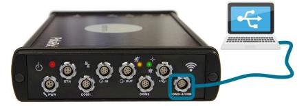
Figure 3-3: Connecting to the front-panel USB socket
