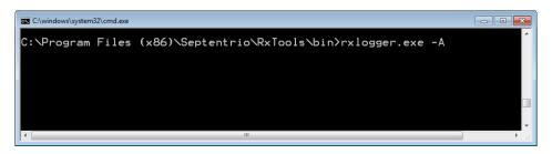
RxLogger can be launched from the command line, as shown in Figure 5-14.
