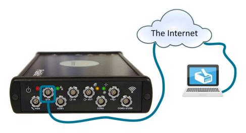
Figure 3-9: Connecting to the front-panel Ethernet socket
