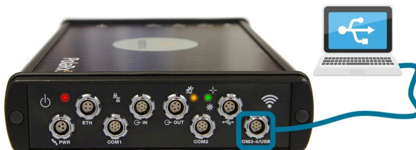
Figure 3-3: Connecting to the front-panel USB socket
