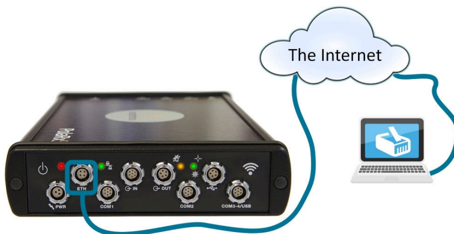
Figure 3-9: Connecting to the front-panel Ethernet socket
