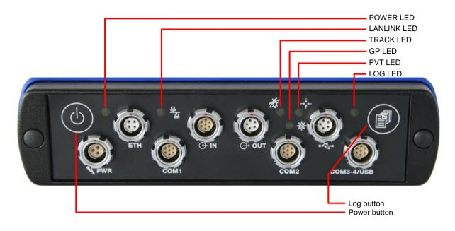
The front panel features 8 ODU connectors, which are described in the following sections. These connectors are all of type ODU MINI SNAP Series F. The pinout of the female connectors and the ODU part number of the corresponding male connectors is shown below.
