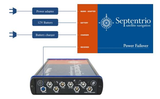
In normal operation, the receiver is powered from the power supply connected to MAINS – ADAPTER. When the voltage at that connector drops below 10.8V, the receiver is powered from the battery instead. A charger is permanently connected to the CHARGER input to charge the battery when the battery is not used to power the receiver.
