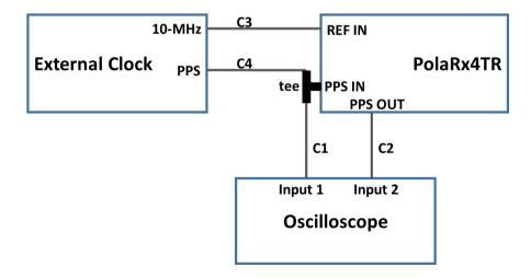
Before measuring the delay, the PolaRx4TR has to be configured to synchronize its PPS OUT signal with the measurement latching epoch. This is done by setting the *TimeScale* argument of the **setPPSParameters** command to "RxClock". You can do this using RxControl (go to the *Navigation* > *Receiver Operation* > *Timing* menu):
