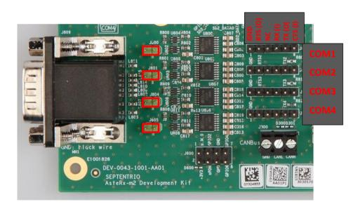
Note that, when using the DB9 connectors, the baud rate must not be larger than 230400baud. This limitation does not apply to the TTL signals.
