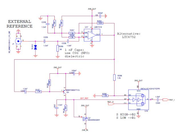
With the above circuit, the module uses the external 10-MHz reference provided at the EXTERNAL REFERENCE connector if a suitable signal is detected. In the absence of external reference, it enables its internal reference. More specifically:
