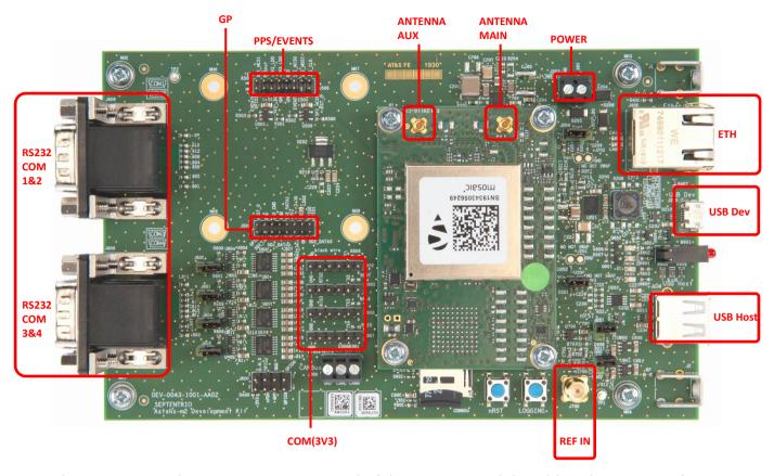
The mosaic Development Kit is composed of the mosaic module soldered on an interface PCB (GTB-0051), itself plugged on the DevKit board (DEV-0043).
