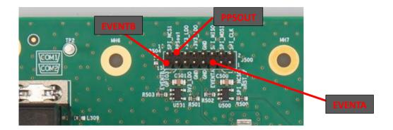
The PPSout pin of header J500 (2x8 2mm-pitch DIL) is connected to the PPSO pin of the mosaic module through a 1.8V to 3.3V level shifter. The PPS level at the header is 3.3V.
