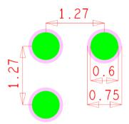
The GND and VDD\_3V3 pins are an exception in this respect. They can be solder mask defined, allowing to route them using a plane.
