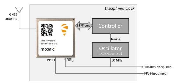
Before use, configure the mosaic so that it starts-up with the PPS pulses disabled, and that it performs an initial precise synchronization to GNSS time. This is done by entering the following user commands:
