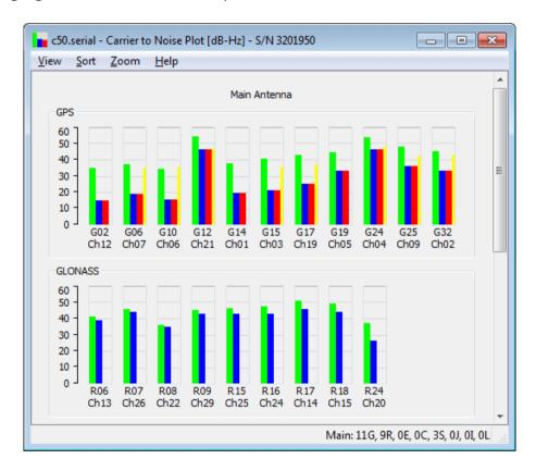
If the maximum C/N0 is lower than expected, interference and cross-talk from nearby electronics is likely, and the source of the problem needs to be identified. This is where the RF spectrum monitor built in the GNSS receiver comes in handy. The spectrum monitor can be accessed in RxControl under the *View / Spectrum View* menu. The spectrum can also be monitored offline if the BBSamples SBF blocks are logged.
