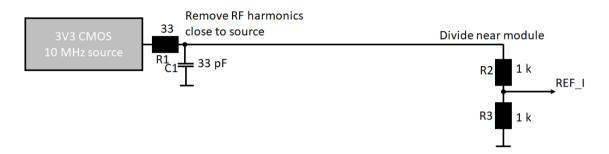
When using an external frequency reference, the internal TCXO is turned off and all time bases in the module are driven by the external reference. In particular, the clock drift reported in the PVTCartesian or the PVTGeodetic SBF block refers to the external clock. It corresponds to the frequency offset of the external reference compared to GNSS time.
