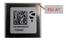
The 2D barcode contains the module variant, hardware version and serial number, e.g.
