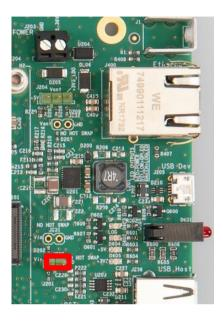
To measure the power consumption of the mosaic module (excluding the contribution from the DevKit and the antenna, but including a small contribution from the interface board, remove the jumper on J200 and connect the two pins to the probes of a multimeter in current-sensing mode. Measure the current flowing between the two pins and multiply it by 3.3V to obtain the power consumption. It is recommended to set the multimeter in high ampere setting to keep the voltage drop as low as possible.
