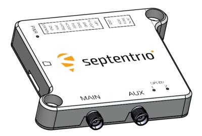
The mosaic-go is composed of the mosaic module soldered on an interface board inside a metallic housing. It serves as an evaluation kit for the mosaic module.
