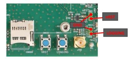
Pressing the nRST button drives the nRST pin of the mosaic low, which resets the module.
