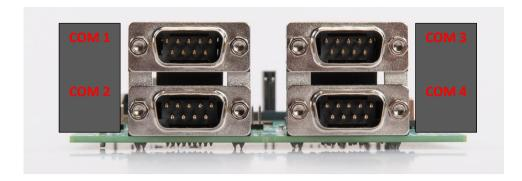
By default, the four COM ports of the mosaic module are routed to the four DB9 connectors of the DevKit. Electrical levels on the BD9 conform to the RS232 standard. RTS/CTS lines are supported only on COM2 and COM3 (the mosaic has RTS/CTS lines on COM1 as well, but they are not routed to the DevKit). Connection to a PC is done through a null-modem cable.
