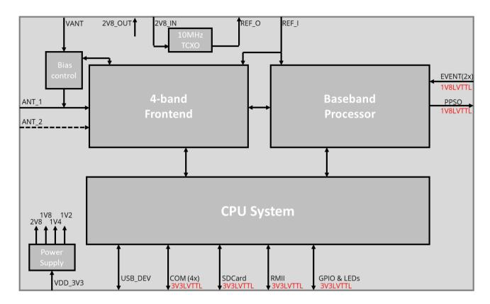
The module operates from a single 3V3 power supply (VDD\_3V3).
