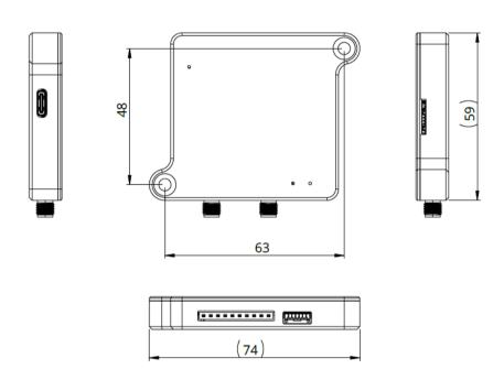
All dimensions in mm. Mounting bolt size = M4.
