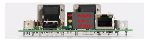
The POWER LED lights when the DevKit is powered.
