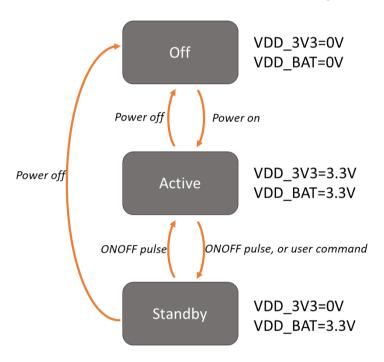
When off, the module is completely turned off. In active state, it is operating with all functions active. Standby state is similar to off, the main difference being in the transition from the active state:
