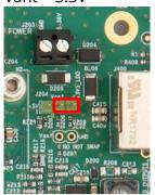
The jumper can be removed if the antenna does not need to be powered by the module. In that case, there is no DC voltage at the antenna connector.
