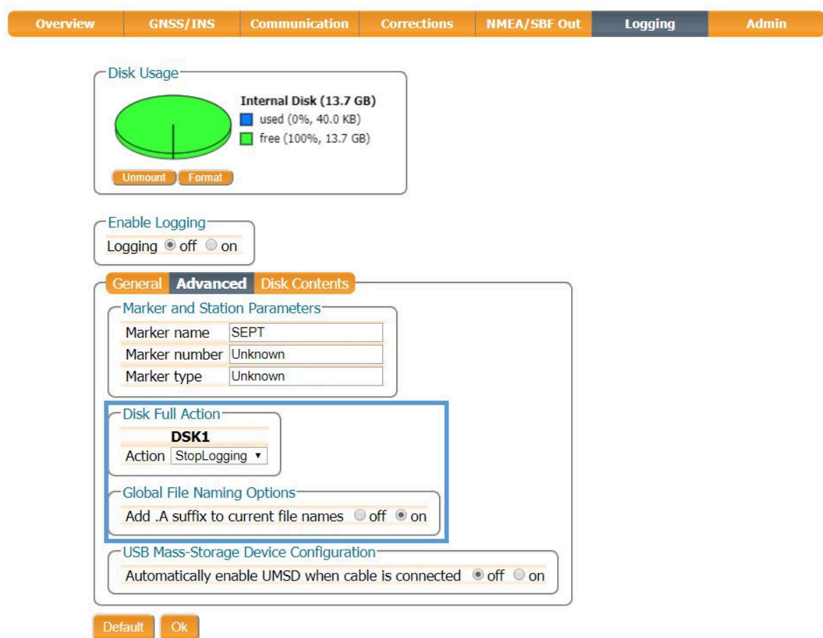
Figure 4-12: Selecting what you wish to happen when the internal 16 GB memory is full
