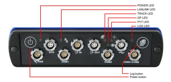
The front panel features 8 ODU connectors, which are described in the following sections. These connectors are all of type ODU MINI SNAP Series F. The pinout of the female connectors and the ODU part number of the corresponding male connectors is shown below.
