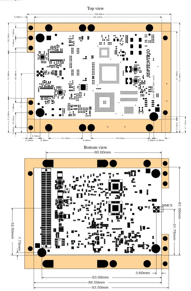
Pin#1 of the 80-pin connector is at the bottom left (marked by the light-gray circle) in the above drawing. Pin#2 is at the bottom right.
