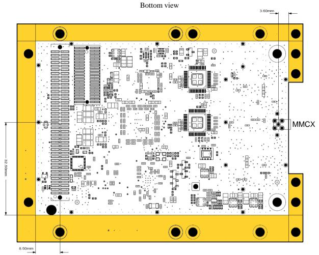
Pin#1 of the 80-pin connector is at the bottom left (marked by the light-gray circle) in the above drawing. Pin#2 is at the bottom right.
