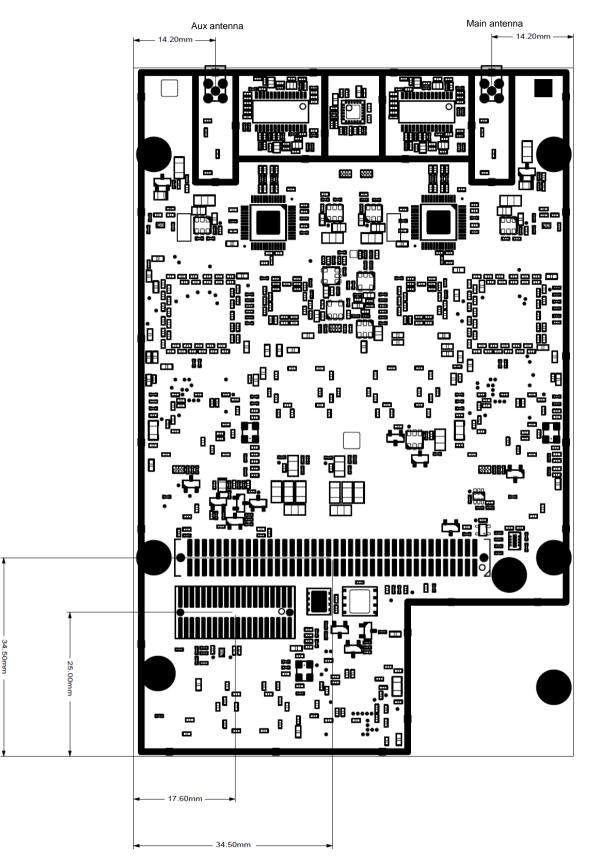
Pin#1 of the 80-pin connector is at the bottom right (marked by the light-gray circle) in the above drawing. Pin#2 is above pin#1. Pin#3 is at the right of pin#1 and so on.
