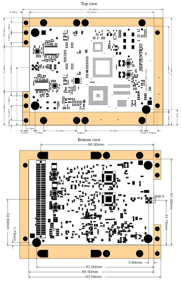
Pin#1 of the 80-pin connector is at the bottom left (marked by the light-gray circle) in the above drawing. Pin#2 is at the bottom right.
