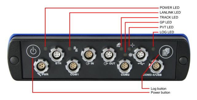
The front panel features 8 ODU connectors, which are described in the following sections. These connectors are all of type ODU MINI SNAP Series F. The pinout of the female connectors and the ODU part number of the corresponding male connectors is shown below.
