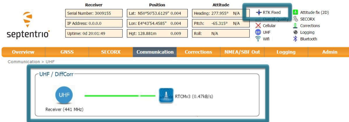
Figure 4-3: The AsteRx-U in RTK mode using differential correction data from a base station transmitting over a UHF radio connection
