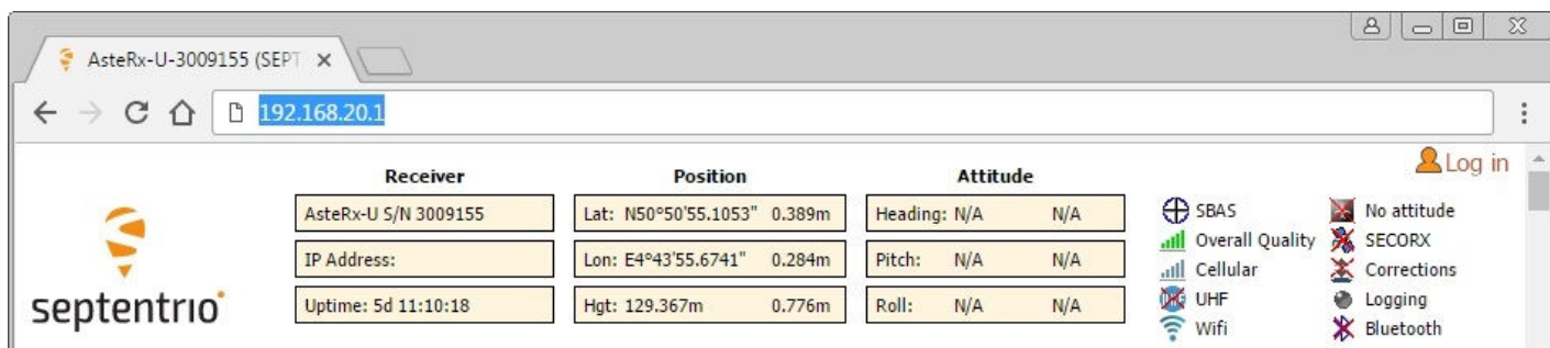
Figure 3-9: Connect to the Web Interface of the AsteRx-U over WiFi using the IP address 192.168.20.1 on any web browser
