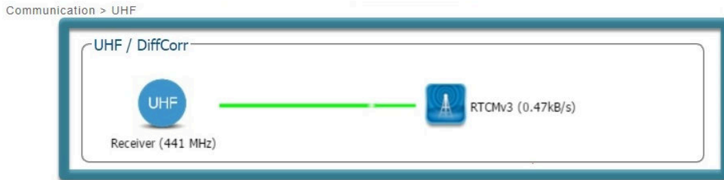
Figure 4-3: The AsteRx-U3 in RTK mode using differential correction data from a base station transmitting over a UHF radio connection
