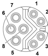
Figure 9-2: 8-pin female socket pin-numbering guide as viewed end on.
