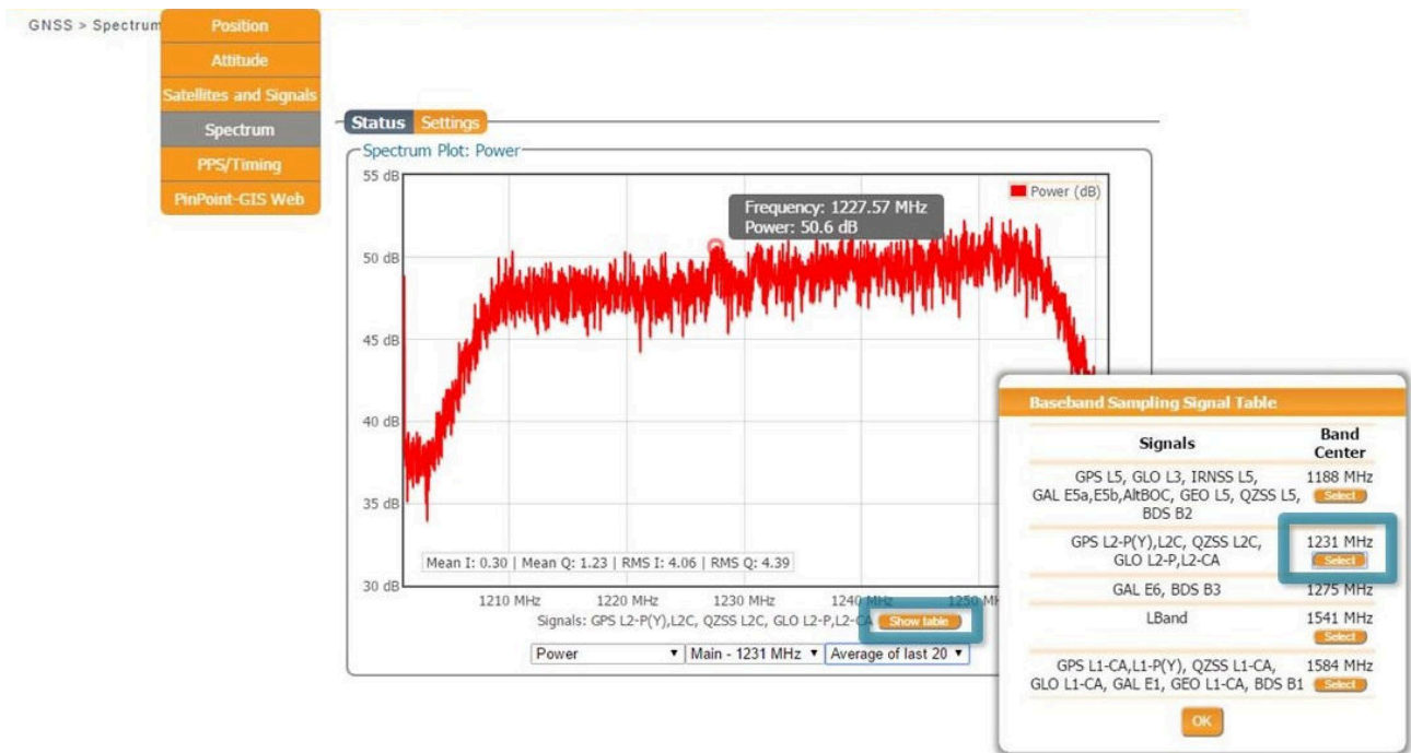
Figure 6-2: The RF spectrum of the L2 Band
