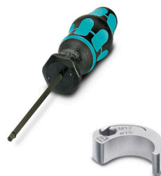
Figure 2-4: Phoenix Contact TSD 04 SAC torque screwdriver, with preset torque of 0.4Nm and 4mm hexagonal drive and SAC BIT M12-D15 for use with M12 connectors
