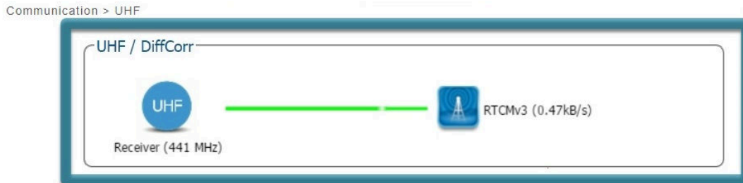
Figure 4-3: The AsteRx-U3 Marine in RTK mode using differential correction data from a base station transmitting over a UHF radio connection
