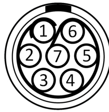
Figure 9-3: 7-pin female socket pin-numbering guide as viewed end on. Start counting at pin indicated by bold semi-circle and follow the line in an anti-clockwise direction. This socket can be paired with a LEMO multipole male connector of type 0B.
