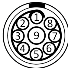
Figure 9-4: 9-pin female socket pin-numbering guide as viewed end on. Start counting at pin indicated by bold semi-circle and follow the line in an anti-clockwise direction. This socket can be paired with a LEMO multipole male connector of type 0B.
