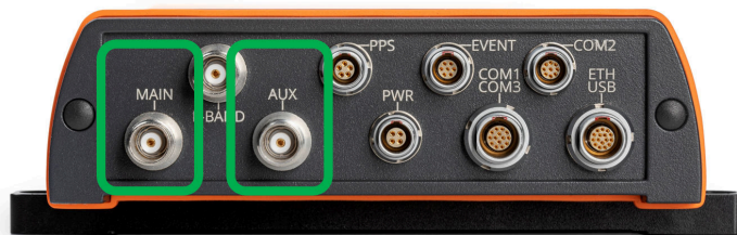
Figure 3-2: Rear-panel main and auxiliary antenna connectors
