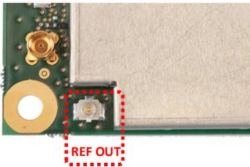
The frequency reference used by the receiver is available at the REFOUT u.FL connector. The signal on this pin provides a 10MHz square wave between 0 - 2.8 V with a 50 Ohm impedance.
