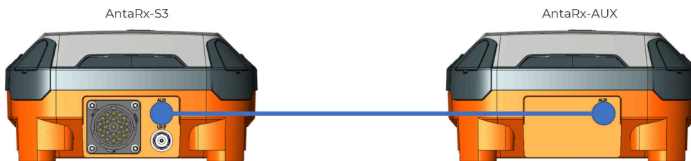
Figure 4-11: Auxiliary antenna connection
