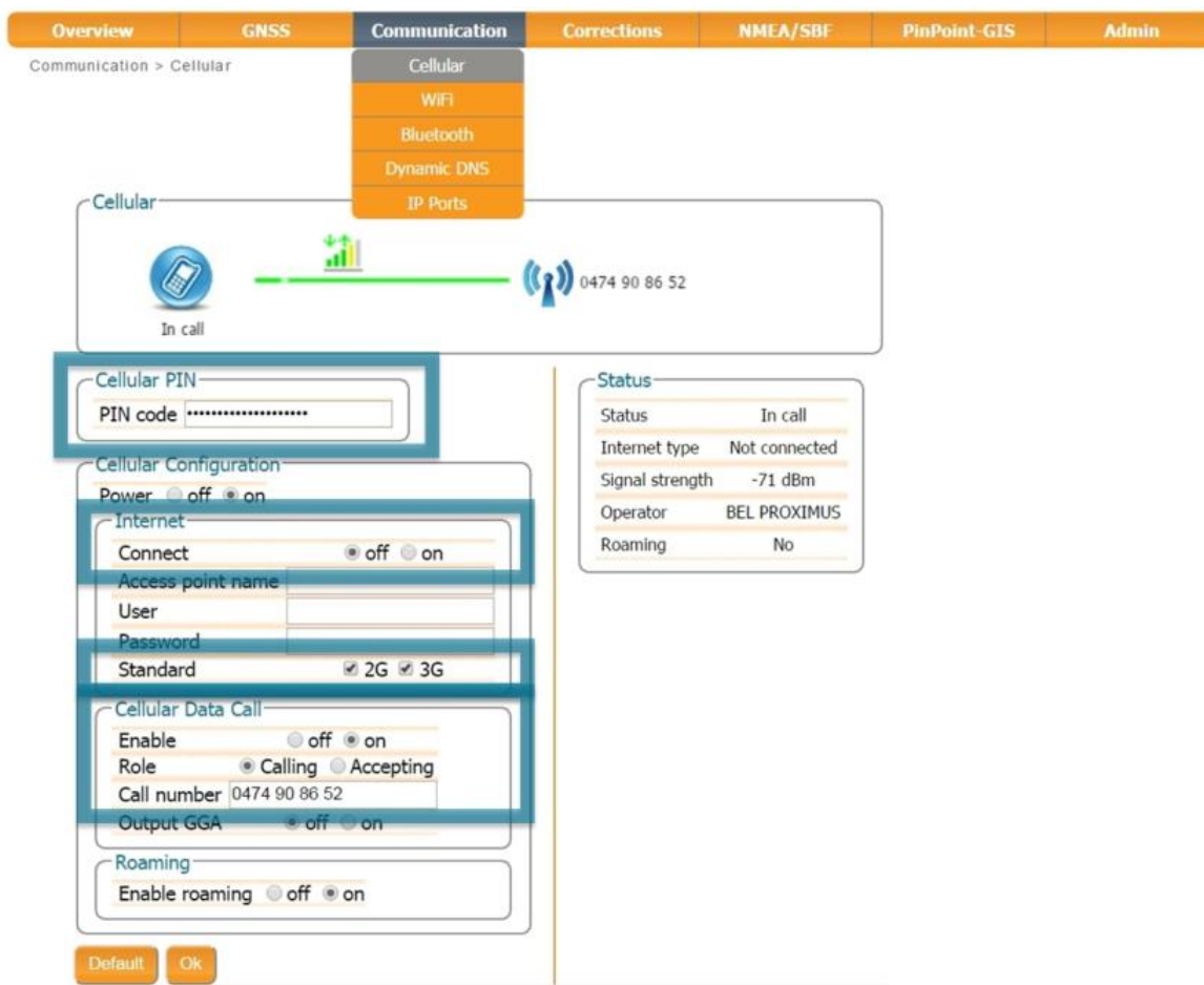
Figure 4-7: Configuring the Base station receiver to receive a data call from the rover receiver
