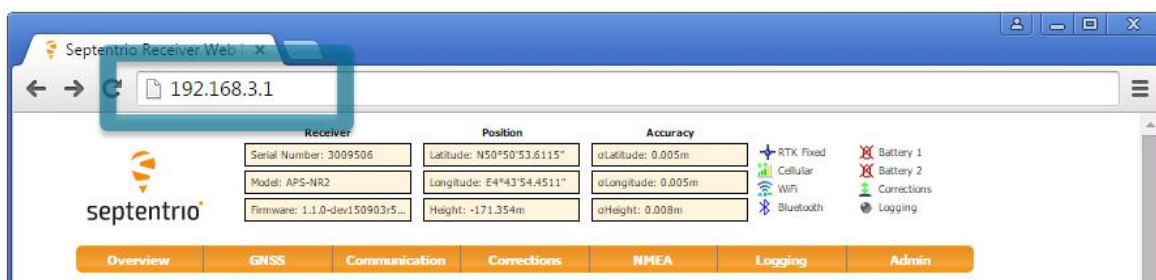
Figure 5-11: Connecting over USB to the web interface using the URL 192.168.3.1
