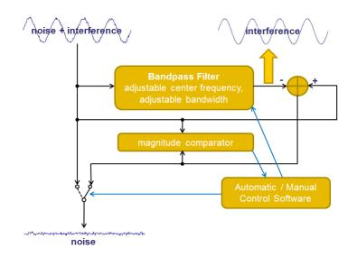
A conceptual diagram of the adaptive notch filter is shown below.
