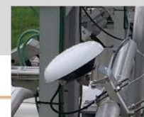
FIGURE 4: The dual-antenna AsteRx-U receiver setup above a 3-lane highway. The antennas were angled forward towards the oncoming traffic to be able to differentiate direction of travel.
